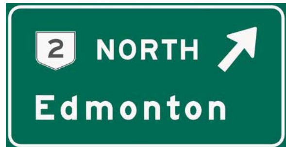
Figure 5.3 – Exit Direction Sign
