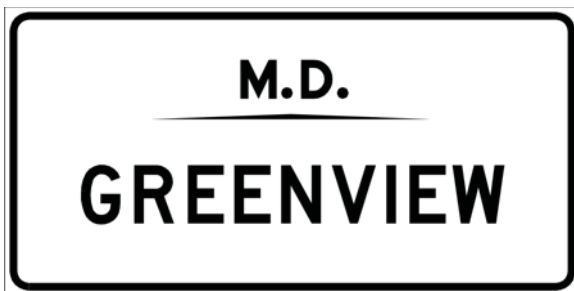
Figure 5.34 – Municipal District Boundary Sign
