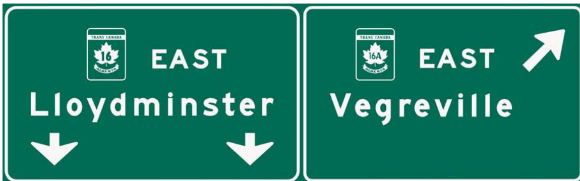
Figure 5.15 – Bypass Route (Single Exit)
