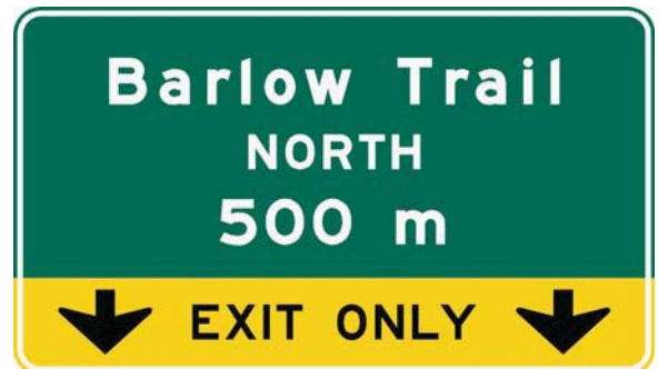
Figure 5.8 – EXIT ONLY - Double Lane Advanced Guide Sign
