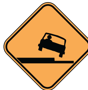
Pavement Drop Off
