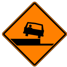
TC-49 PAVEMENT DROP-OFF
