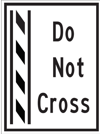
HOV – DO NOT CROSS LEFT Sign (Ground-mounted) (HOV-4aL)
